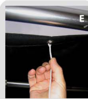
Use one half of line for each half of the top. Take the line from under the top and put it up through the eyelet.
