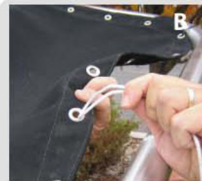
Fold length of line in half, and put over the pipe and through eyelet.
